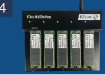
When each target port green light is steady indicates the copy process has been completed. The red light turns on when a SSD fails to copy.
